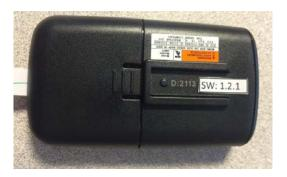
The "SW: 1.2.1" marking indicates that the most recent circuit board is in inside the remote.
