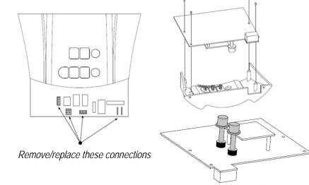
The only added steps from the board with the plastic to the new part number is to remove 4 screws attaching the plastic to the board, gently pulling the antenna wire through and removing and reinserting force control shafts from the original board onto the new board.
