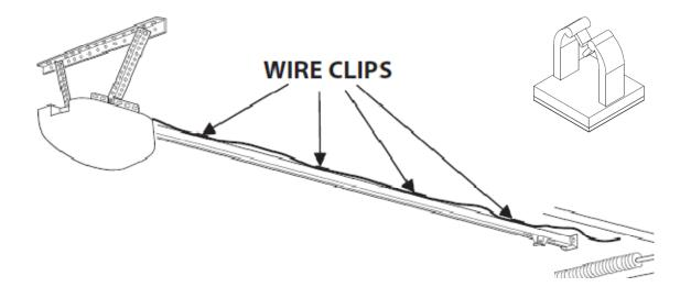
(Remove adhesive pad on the bottom of the clip and adhere to rail surface)
