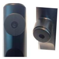
**Spring 2016** – The tube was lengthened and the beam was narrowed to help reduce nuisance reversals caused by light infiltration.
